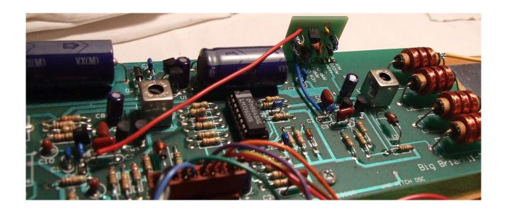
C2 is aimed differently. The 'var' wire is connected to the leg that is closest to the centre of the etherwave circuitboard.
