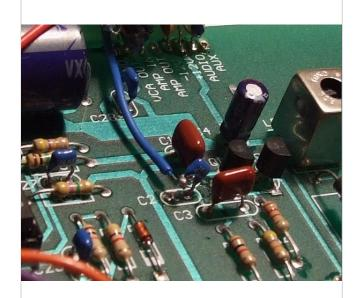
C6 is located all the way to the lefthand side of the circuitboard. The bare wire connected to the 'fix' position on the module is not long enough. It needs to be replaced with a longer, coated wire. It should be coated as it will touch the large ELCO on its way to C6.
