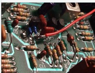
There is an alternative way to connect to C6, using the traces of the Etherwave itself. Following the image below, make a bridge between resistor R23 and diode D4. Solder the fix wire to either of the freed up holes.
